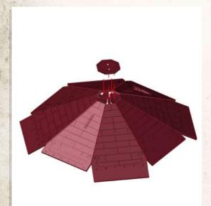
NOTE: The roof tiles go round in a circle alternating between the longer and smaller versions, using the octagon piece to help hold them together
