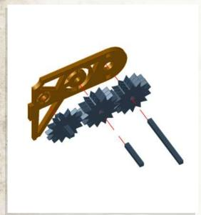
NOTE: Allow gears to rotate freely
