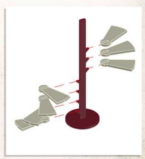
NOTE: Glue the steps numbered 1-7 from the bottom, up, with the numbers facing down to be hidden
