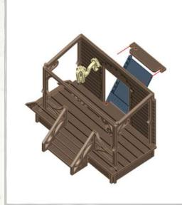
NOTE: Fit the door between the two door hinge holes without glue
