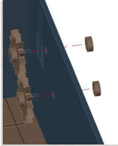
NOTE: DO NOT glue gears to wall, allow them to rotate freely
