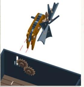
NOTE: Align gears, they should all rotate freely
