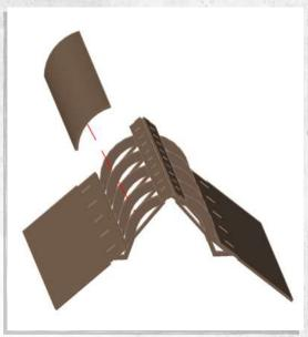
NOTE: Carefully bend the MDF hinge around the beams
