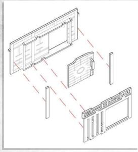
NOTE: Place the door within the frame (DO NOT GLUE) to allow it to slide. NOTE: Repeat for mirrored version.
