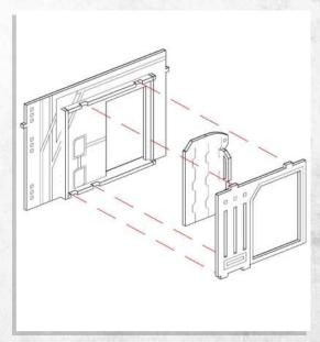
NOTE: Use Parts Labeled 'B'. NOTE: Place the door within the frame (DO NOT GLUE) to allow it to slide.
