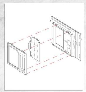
NOTE: Use Parts Labeled 'A'. NOTE: Place the door within the frame (DO NOT GLUE) to allow it to slide.
