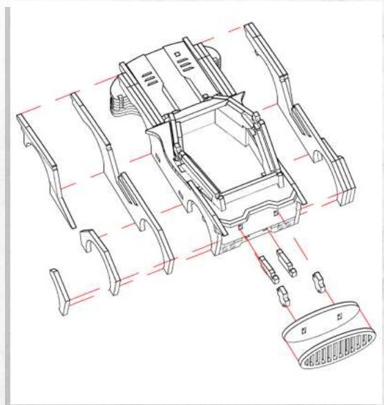
**NOTE:** Insert but **DO NOT GLUE** the bonnet into the hinge holes.
