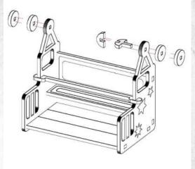
NOTE: Only glue one screw in place on one side of each carriage.
