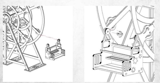
NOTE: Use the screw that's glued in place to line up the placement of the carriage, then glue another screw into the other side of the carriage to fix it in place. Repeat these two steps for all six carriages
