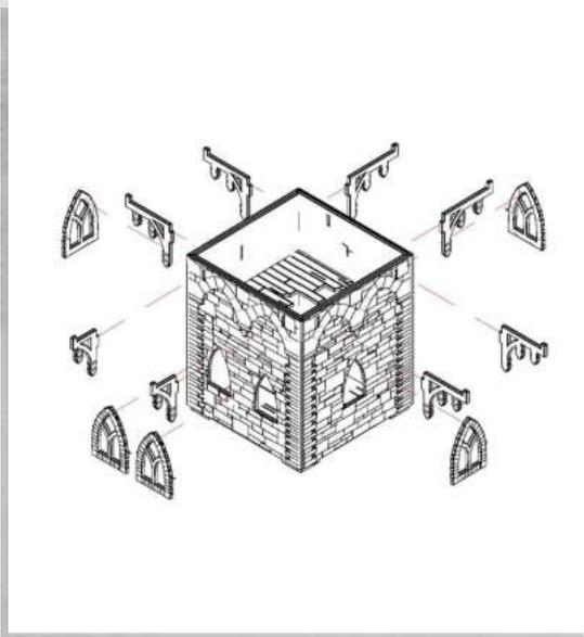
NOTE: Glue the shortest brackets to the double-windowed wall and the longest brackets to the opposite back wall
