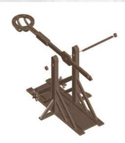
NOTE: Thread the bar through the middle before gluing the outside pieces
