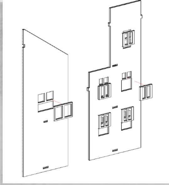
NOTE: Glue all windows on the inside of the four walls. Each window piece can be glued at different heights; examples shown above
