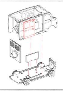
NOTE: Slide in the doors without gluing. Ensure the side door is aligned with the roof sliders.
