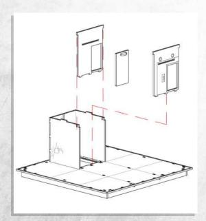
NOTE: Sandwhich the door between the two panels.
