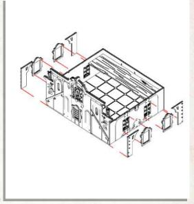
NOTE: Line up parts G21 with the bottom edge of D5/E5
