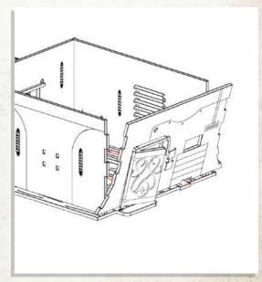
NOTE: Glue the wall while fitting the door in place. Do not use glue on the door
