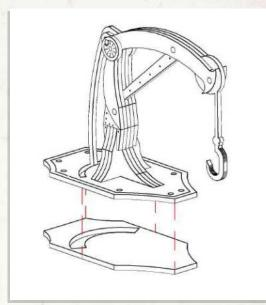
NOTE: Do not use glue near the extended foot. The crane can now be rotated to different positions
