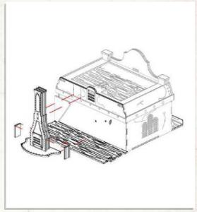
NOTE: Align the chimney with the vertical lines on the back wall
