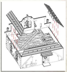
NOTE: Using I3 as a placement guide, glue the base of G5 parts to the roof
