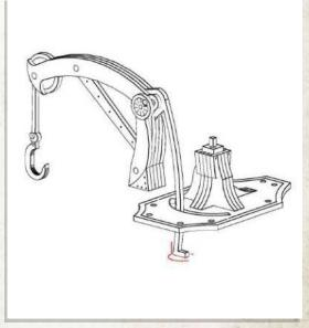
NOTE: Do not use glue. Fit the extended foot through the gap in the floor plate, then rotate and lift the crane back up
