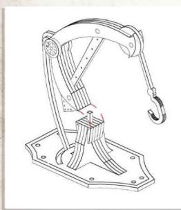
NOTE: Do not use glue. Fit the crane on top of the base, keeping the extended foot under the floor plate
